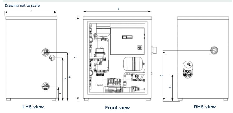
Unit must be installed at least 100mm away from a solid surface to enable the type 'AB' airbreak to function correctly at the back of the unit.
